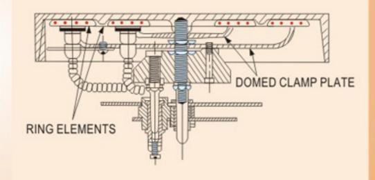
If the utensil is having thick bottom, The mounting of the element is very simple. A centre bolt & a concave fixing plate alone being necessary, as shown.
