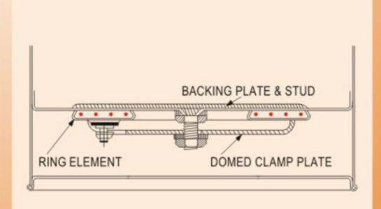
If the utensil bottom is thin, we suggest to strengthen it by means of brass / SS backing plates which makes one piece with the fixing bolt mounted as shown.
